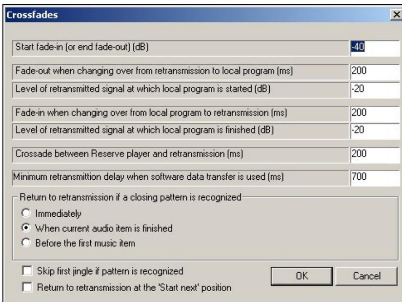
Fig. 8. Setting of crossfades in the window **Crossfades**
